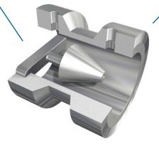
The Wafer-Cone flow meter is available in line sizes from 1 to 6 inches and can be oil or gas flow calibrated. Featuring a removable cone and flangeless design, cones with different beta ratios can be easily exchanged to accommodate changing flow conditions without the need for recalibration.
