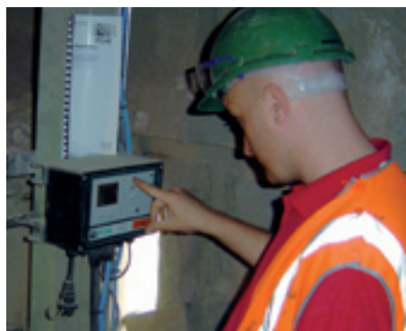
PCME instruments offer easy set-up/ interrogation of monitors either locally or remotely by either modbus /4-20mA outputs or via Ethernet, GSM & Web connectivity
