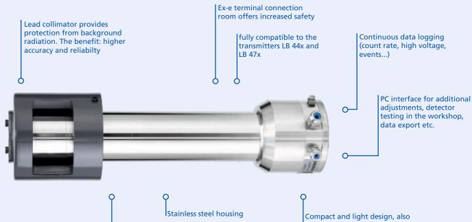
Improved water cooling, covers the entire detector and can also be retrofitted Compact and light design, also ideally suited for the use in dip pipes.
