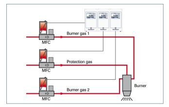
Burner control using Mass Flow Controllers brings many advantages compared to conventional systems, where flow is adjusted through needle valves. When burner orifices get clogged or when gas supply pressure varies, an MFC will automatically adapt to the changed conditions. For the control of relatively large flows with low differential pressure, which is typical for natural gas or CH<sub>4</sub>, Bronkhorst offers mass flow meters with separate pressure compensated bellows valves.
