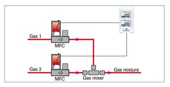
MFC's are often used to make precise and stable mixtures of two or more gases. A Bronkhorst<sup>®</sup> PS/Readout system can be applied to maintain the ratio of mixed gases by operating in master-slave mode. In the example above, the flow range of gas 1 is much smaller than the other. For this purpose Bronkhorst developed a gas mixer, to guarantee a homogeneous gas mixture.
