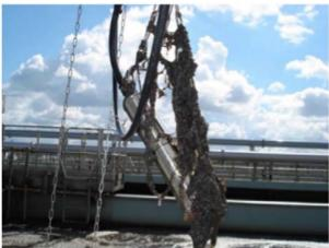
contamination is apparent but the measuremet gap was not clogged, which is due to the automatic cleaning by compressed air. For this reason, the cleaning takes only a few minutes and the device can be put back into operation after a short time.
