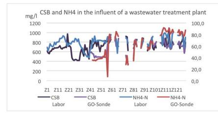
the influent of a wastewater treatment plant. In The first half the values measured by the ISA and in the laboratory are very different, very large meandering are visible. But from sample Z50 to the last sample (Z91) the values become more similar in both ammonium and COD. The reason for that is, that a good calibration needs as many samples as possible to get correct. Especially NH4 laboratory tests may be influenced by changes in work
