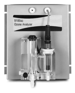
The Hach 9185sc Amperometric Ozone Sensor is free from interference from oxidants such as bromine, chloramines, chlorine, chlorine dioxide, and hydrogen peroxide as well as pH and low-conductivity water. This sensor was designed to meet the specific needs of ozone measurements in drinking water plants, pure water loops, and the bottled water industry
