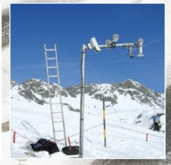
The measurement method of the SHM31 is based on a combination of phase comparison and time of flight. The platform-independent UMB-Config tool enables the parameterization of the sensor according to the individual requirements.
