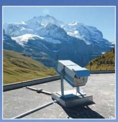
Equipment is required on location to check the functionality. The Lufft cloud height simulator allows ceilometers to be tested, even under a cloudless sky.
