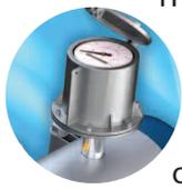
The Mc SpaceSaver Flow Meter comes with a standard instantaneous flow rate indicator and a straight-reading totalizer. Unlike mag and other types of flow meters, the Mc SpaceSaver requires no electric power to operate. With no Lithium batteries to fail in extreme heat or cold or humidity, your valuable flow data is continuously available and safe via the Mc SpaceSaver's standard register.
