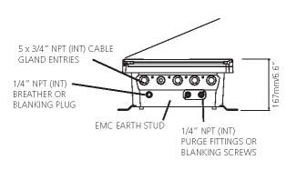
SERVICE ACCESS REQUIRED FOR DOOR TO BE OPENED: 365mm/14.4" IN FRONT 250mm/9.9" TO LEFT HAND SIDE
