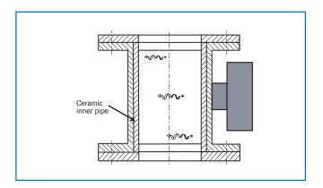
If the material speed varies, for example due to a change in initial speed, then this can also be measured. This takes place through a runtime measurement with the help of two additional electrodes behind the interior ceramics tube.
